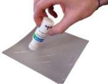
Apply Clean Stick adhesive evenly on the rubber. To do this, press the stick firmly onto the sponge with the sponge applicator attached and distribute evenly.
